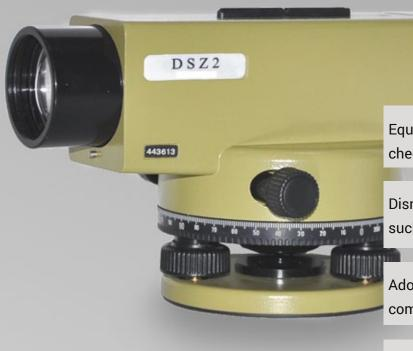
Equipped with a press button for compensator checking.
